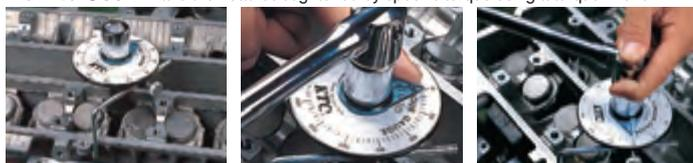
2. Set the angular torque gauge and stop the rotation with L-shape stopper.
