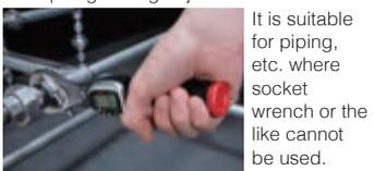
It is suitable for piping, etc. where socket wrench or the like cannot be used.
