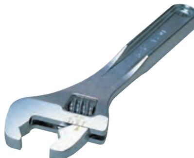
Tightening and loosening Tie-rod end lock nuts
