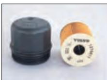
Oil filter cap and replacement filter paper for VOLVO
