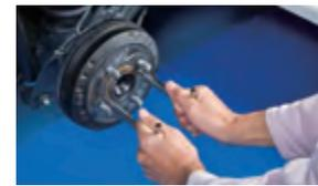
When two handles are used, the brake drum can be removed in a stable manner.
