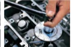
2. Set the angular torque gauge and stop the rotation with L-shape stopper.
