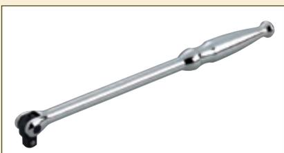
The square drive can bend left or right up to 90° about a pin in the center of the head part of the shank and stop at a given angle. When turning quickly to temporarily tighten and so on, the handle can be held straight and used like a screw driver (Fig. 1), and when tightening securely, a strong torque can be generated by holding the handle to the side (Fig. 2).
