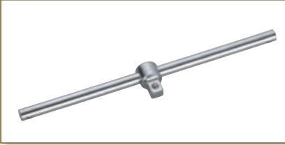
The drive head can be stopped at any place on the handle, and it can be used either as an L shaped wrench or a T shaped wrench. When using as an L shaped wrench (Fig. 1), first pull towards you, and when you have turned 180°, slide the handle and pull the handle towards you again. When using as a T shaped wrench (Fig. 2), set the square drive in the center of the handle and turn with both hands. To make a T wrench with a longer axis, the extension bar is connected (Fig. 3).
